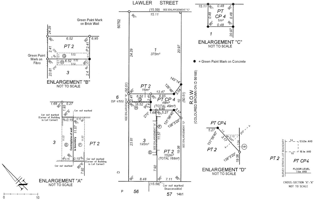
A.H.D Levels Established From S.M.H 1159 Using Data Supplied by the Water Corporation
